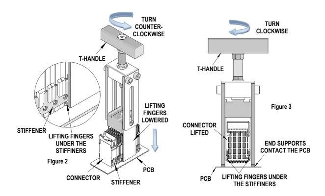
Note: After removing the header assembly from the PCB, some terminals may remain in the board. This is not a tooling malfunction. A pair of needle nose pliers may be used to individually remove the terminals. Caution is required when using this method; if a terminal is incorrectly gripped or pulled away at an angle, it could break off inside the PCB hole. After terminals are pulled out of the PCB, they should be discarded. The PCB should be free of any contact debris.
