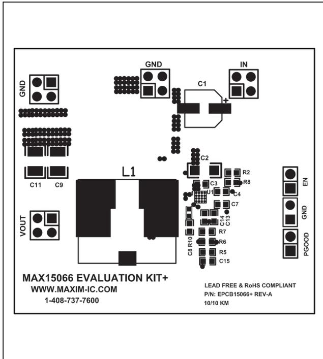
Figure 2. MAX15066 EV Kit Component Placement Guide—Component Side
