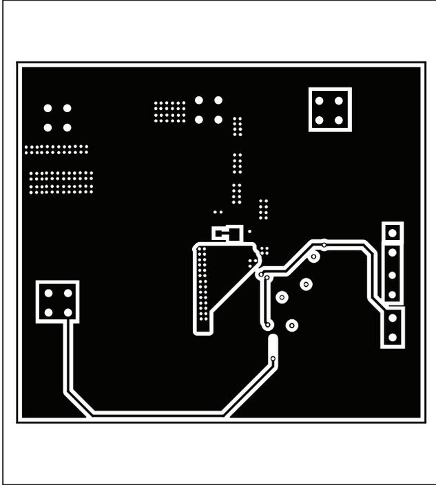
Figure 6. MAX15066 EV Kit PCB Layout—Solder Side
