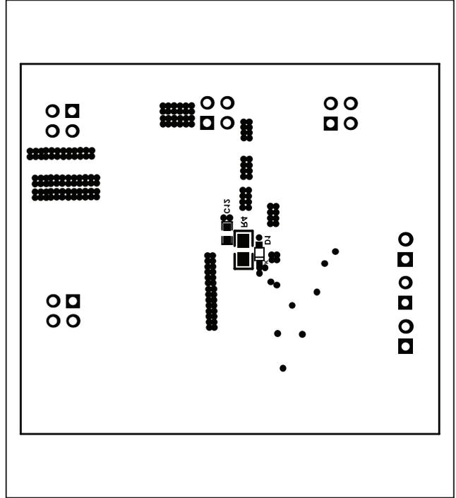
Figure 7. MAX15066 EV Kit Component Placement Guide—Solder Side
