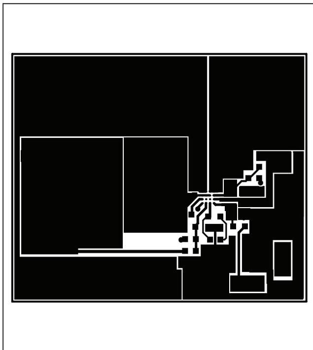
Figure 3. MAX15066 EV Kit PCB Layout—Component Side
