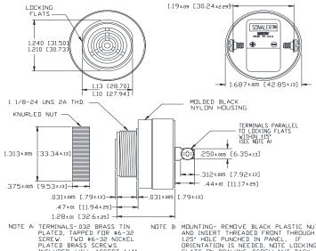
NOTE A: TERMINALS-032 BRASS TIN PLATED, TAPPED FOR #6-32 SCREW. TWO #6-32 NICKEL PLATED BRASS SCREWS INCLUBED. WILL ACCEPT 1/4' QUICK CONNECT.
