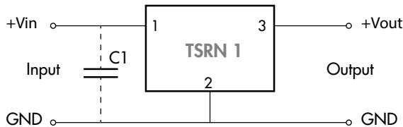
C1 = 22  $\mu$ F / 50 V (required only if input voltage is higher than 36 V)
