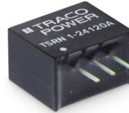
The new TSRN-1 series step-down switching regulators are drop-in replacement for inefficient 78xx linear regulators. A high efficiency up to 95 % allows full load operation up to  $+70^{\circ}\text{C}$  ( $+85^{\circ}\text{C}$  with derating) ambient temperature without the need of any heat-sink or forced air cooling.
