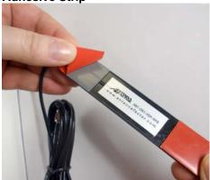
Figure 18. Adhesive Mount Antenna - Step 3. Mount the **Antenna**
