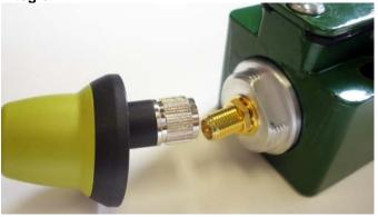
Figure 14. Limitless™ WGLA RP-SMA Connection, Remote
