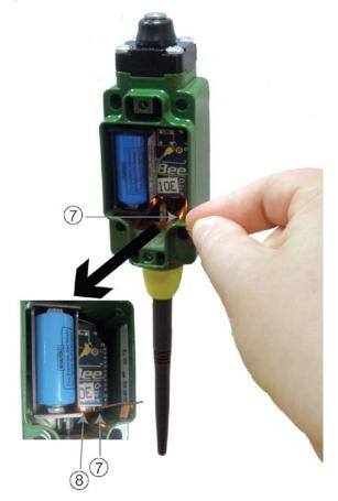
NOTE: Use a blunt object, such as a paper clip or tooth pick to actuate the function switch  $\Im$ .
